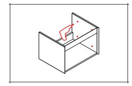
Drill fixing holes in the Basin unit and furniture unit using an appropriate size drillbit for the concealed threaded
