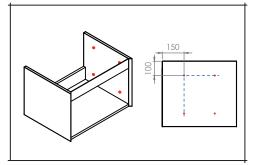
OPTION 1 - Mounting on one side: Mark 4 fixing locations on the carcass of the furniture and the spacer.
